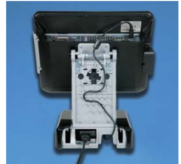
Integrated Power Supply and Cable Management Keeps Cords Hidden and Organized
